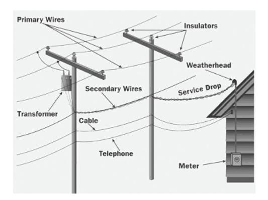
**Important Note:** During or after any storm event, consider all downed wires to be energized and dangerous, including telephone, fiber optic and cable TV wires. They may be in contact with energized electric wires that are not within your view. To report downed electric wires, please call **1-800-867-5222**.
