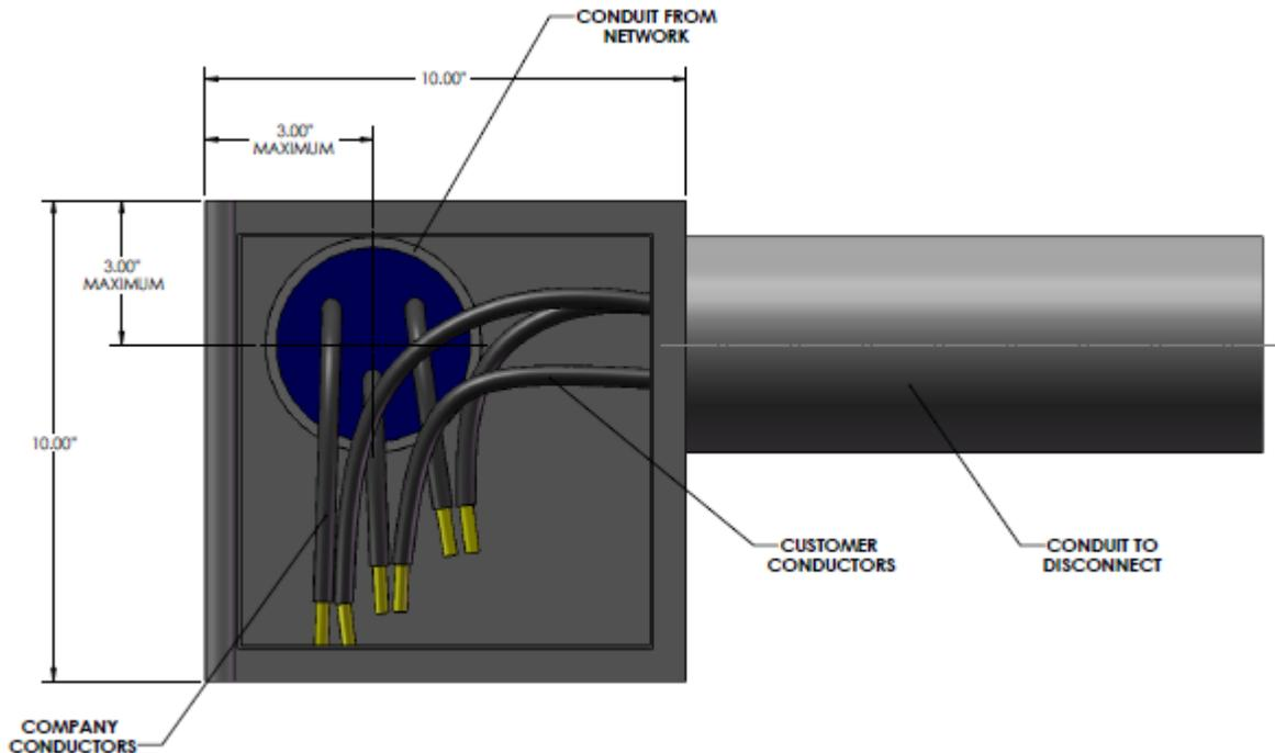
**Figure 4 – Single Phase Junction Enclosure Example Layout with conductors**
