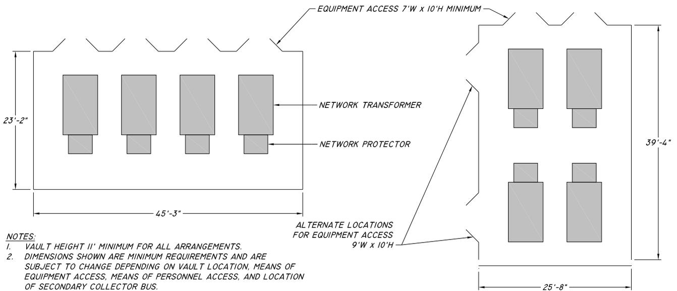
**Figure 28 – Building & Free-Standing Vault Standard Arrangements, 4 – 2500 kVA, 15 kV**
