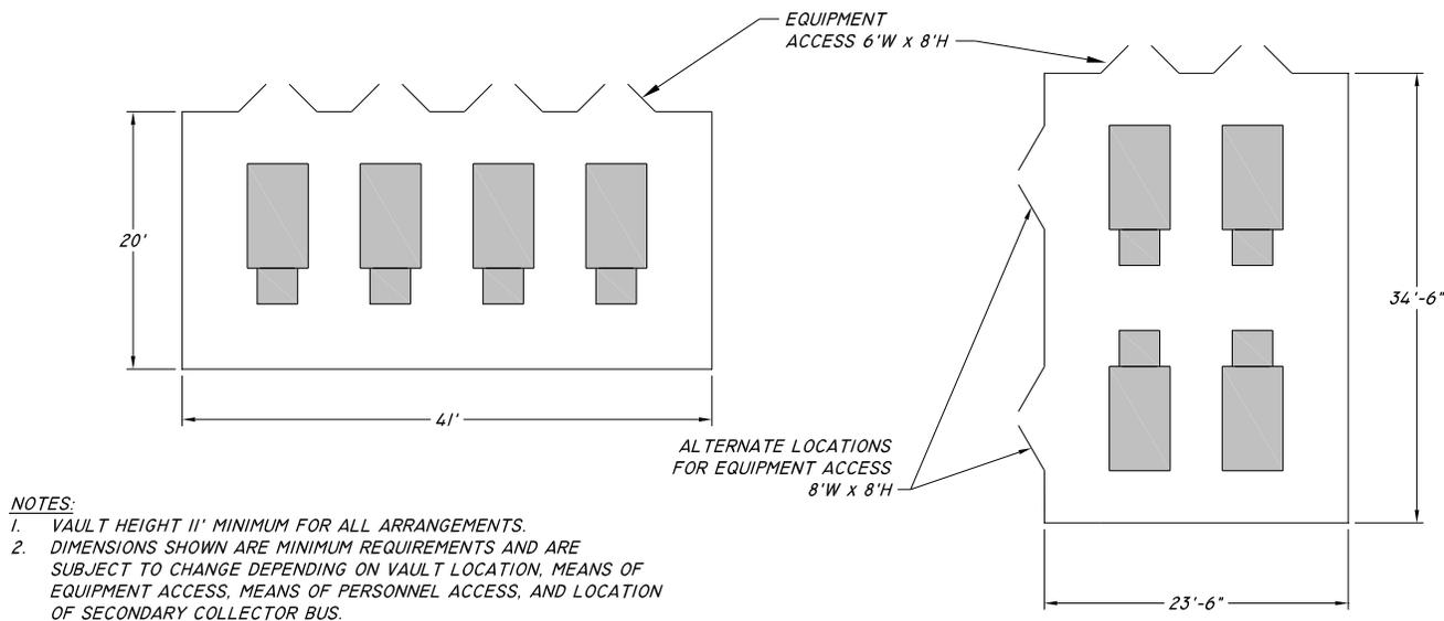
**Figure 22 – Building & Free-Standing Vault Standard Arrangements, 4 – 1500 kVA, 15 kV**
