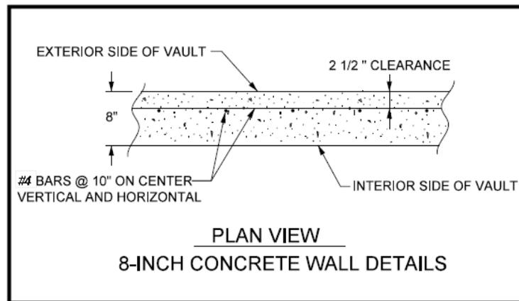
Figure 52 – 8” Concrete Wall Minimum Standards
