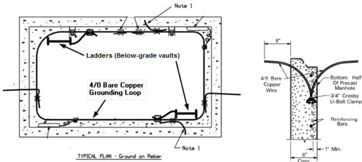
**Note 1** – Minimally two 4/0 tails bonded to vault rebar are required. Additional 4/0 tails may be required for vaults that are cast with separate floor sections. Ground bonding shall connect floor and all wall sections. Epoxy coated rebar is not allowed.
