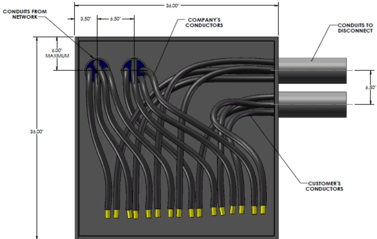
**Figure 10 – 800 ampere Three Phase Junction Enclosure Example Layout with conductors**
