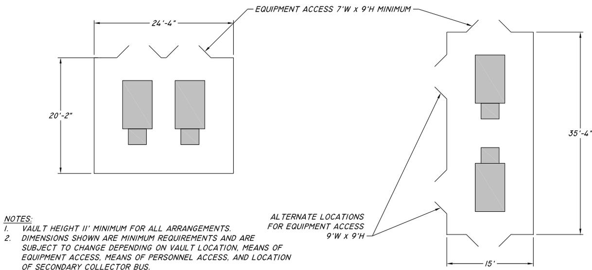
**Figure 32 – Building & Free-Standing Vault Standard Arrangements, 2 – 1500 kVA, 23 kV**
