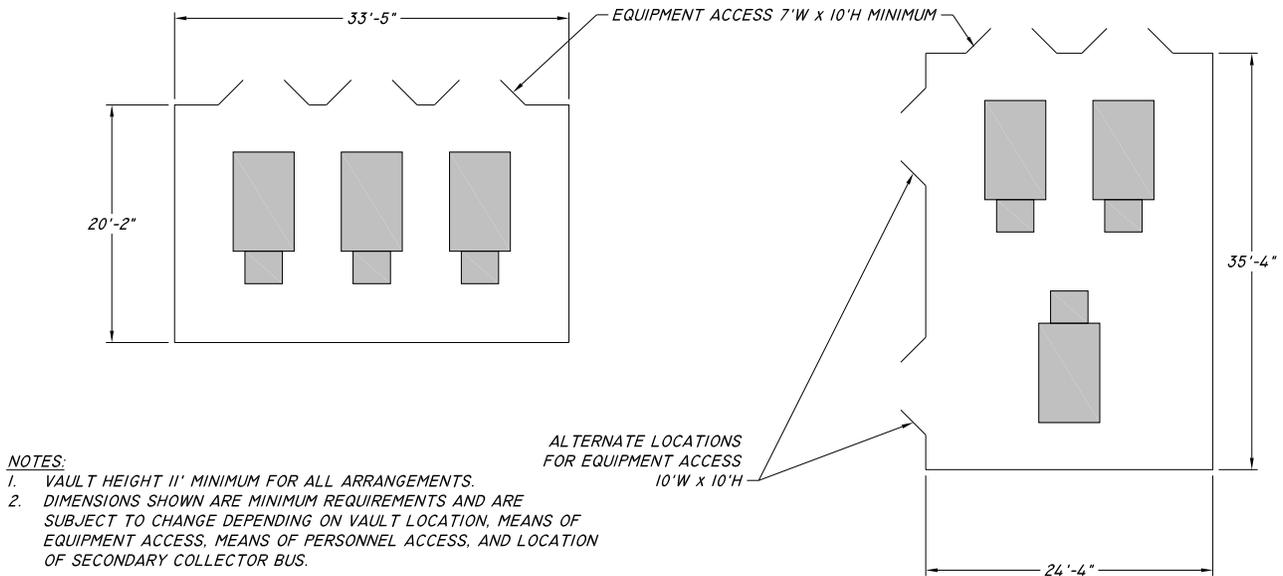
**Figure 33 – Building & Free-Standing Vault Standard Arrangements, 3 – 1500 kVA, 23 kV**
