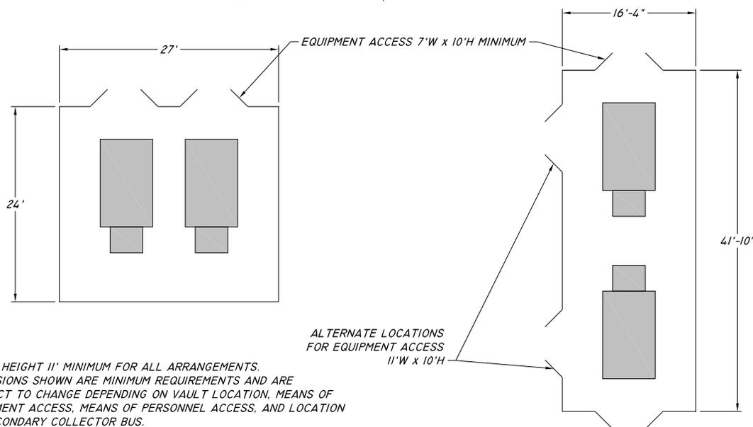
**Figure 38 – Building & Free-Standing Vault Standard Arrangements, 2 – 2500 kVA, 23 kV**
