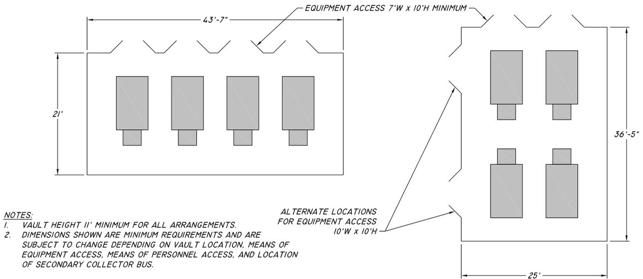
**Figure 43 – Building & Free-Standing Vault Standard Arrangements, 4 – 1500 kVA, 34.5 kV**
