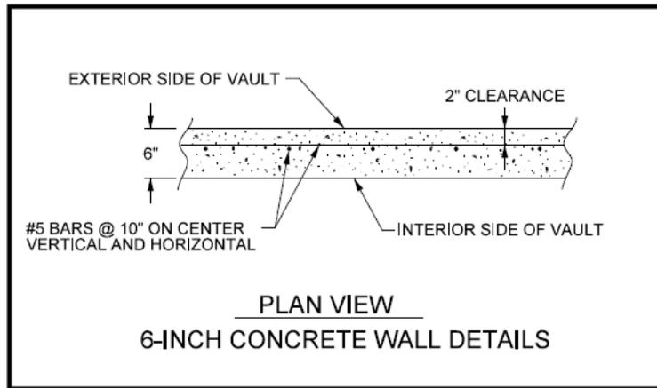
Figure 51 – 6” Concrete Wall Minimum Standards
