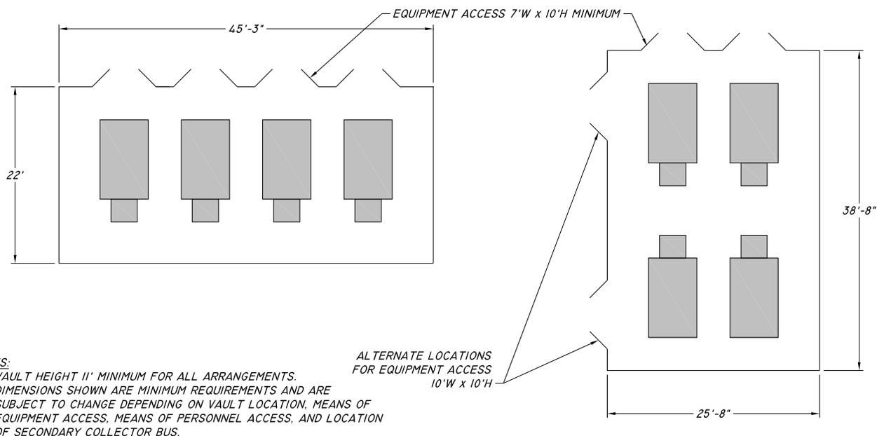
**Figure 37 – Building & Free-Standing Vault Standard Arrangements, 4 – 2000 kVA, 23 kV**
