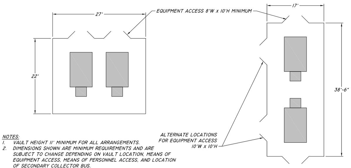
**Figure 44 – Building & Free-Standing Vault Standard Arrangements, 2 – 2000 kVA, 34.5 kV**
