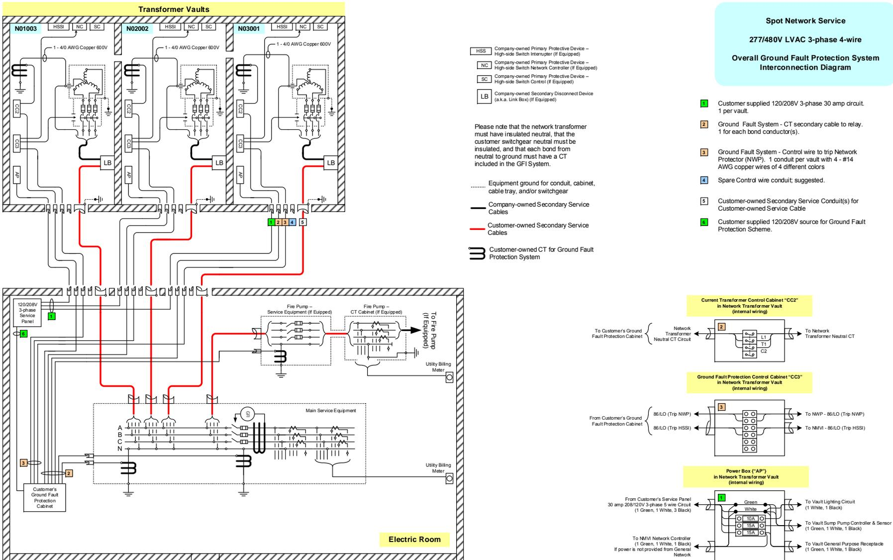
Figure 57 – Ground Fault Protection Interconnection Example
