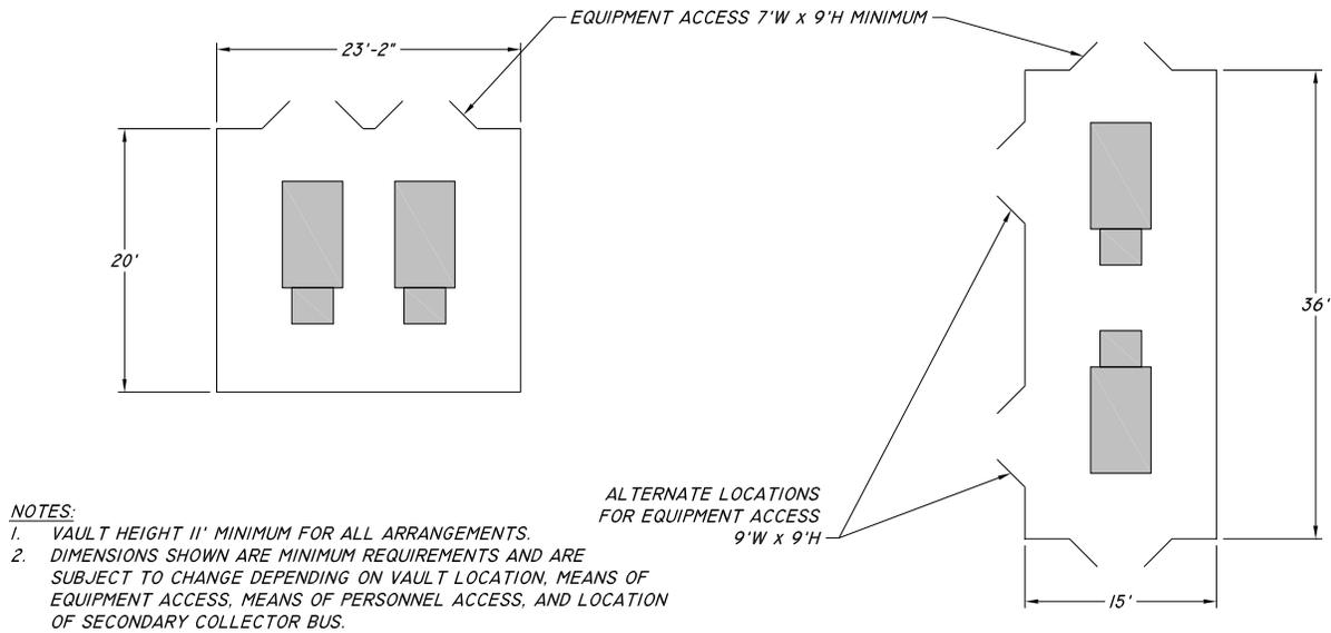
**Figure 29 – Building & Free-Standing Vault Standard Arrangements, 2 – 1000 kVA, 23 kV**
