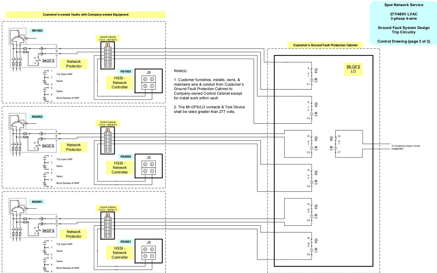
Figure 59 – Ground Fault Protection Control System Example Sheet 2
