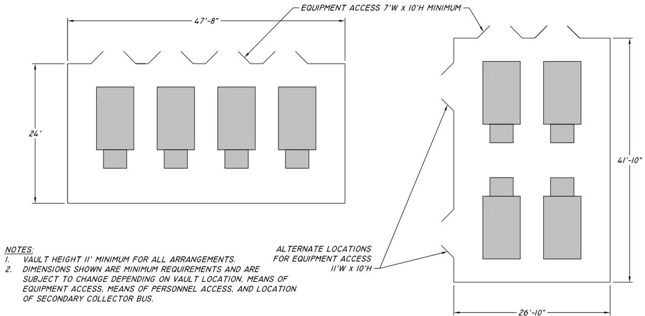
**Figure 40 – Building & Free-Standing Vault Standard Arrangements, 4 – 2500 kVA, 23 kV**
