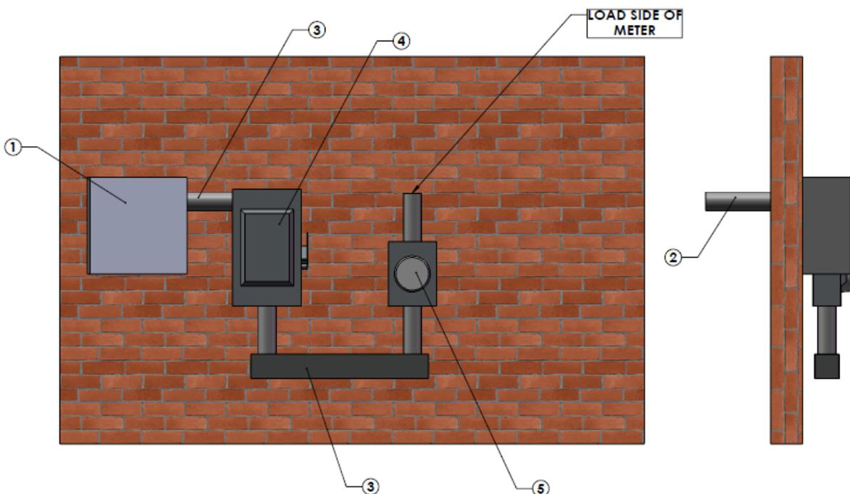
**Figure 5 – 200 ampere Three Phase Equipment Example Layout**
