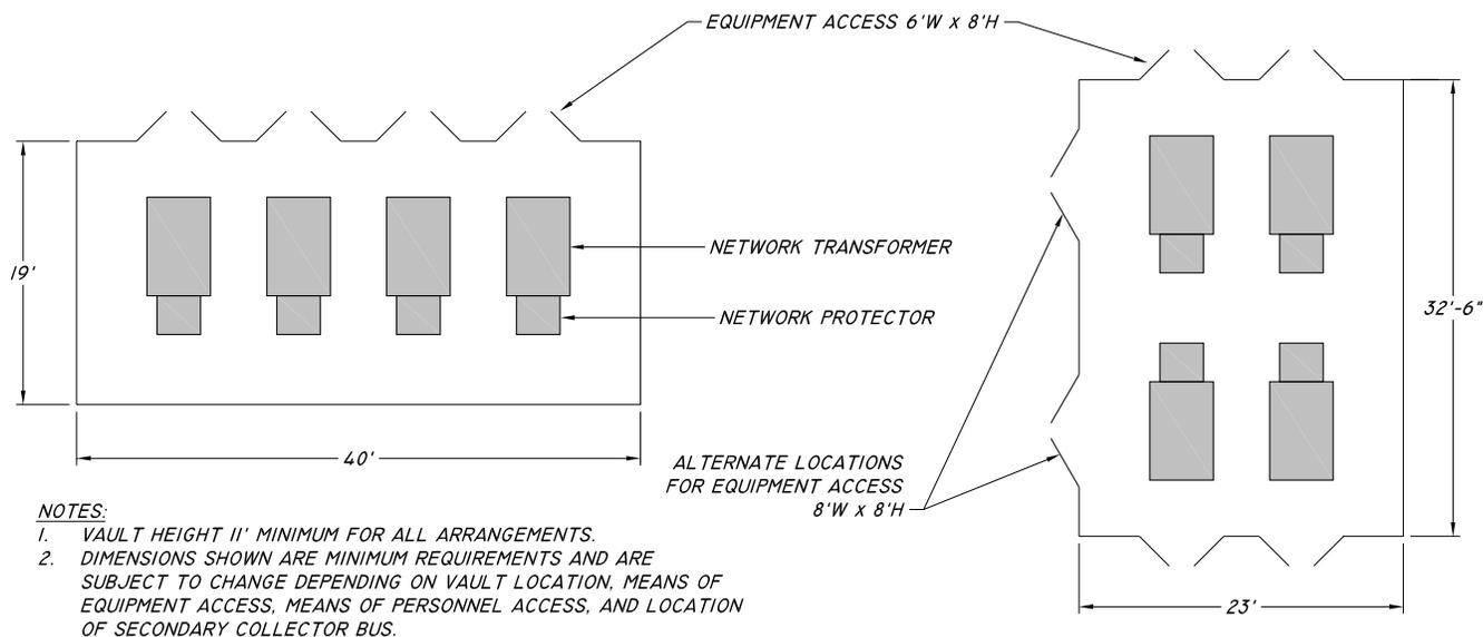
**Figure 19 – Building & Free-Standing Vault Standard Arrangements, 4 – 1000 kVA, 15 kV**
