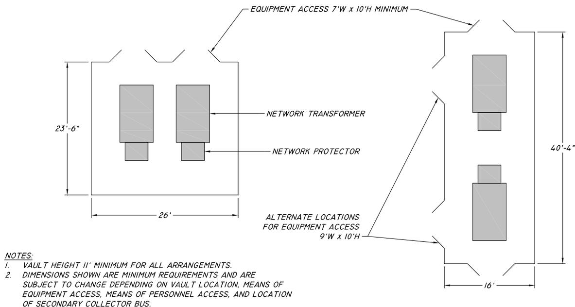
**Figure 26 – Building & Free-Standing Vault Standard Arrangements, 2 – 2500 kVA, 15 kV**
