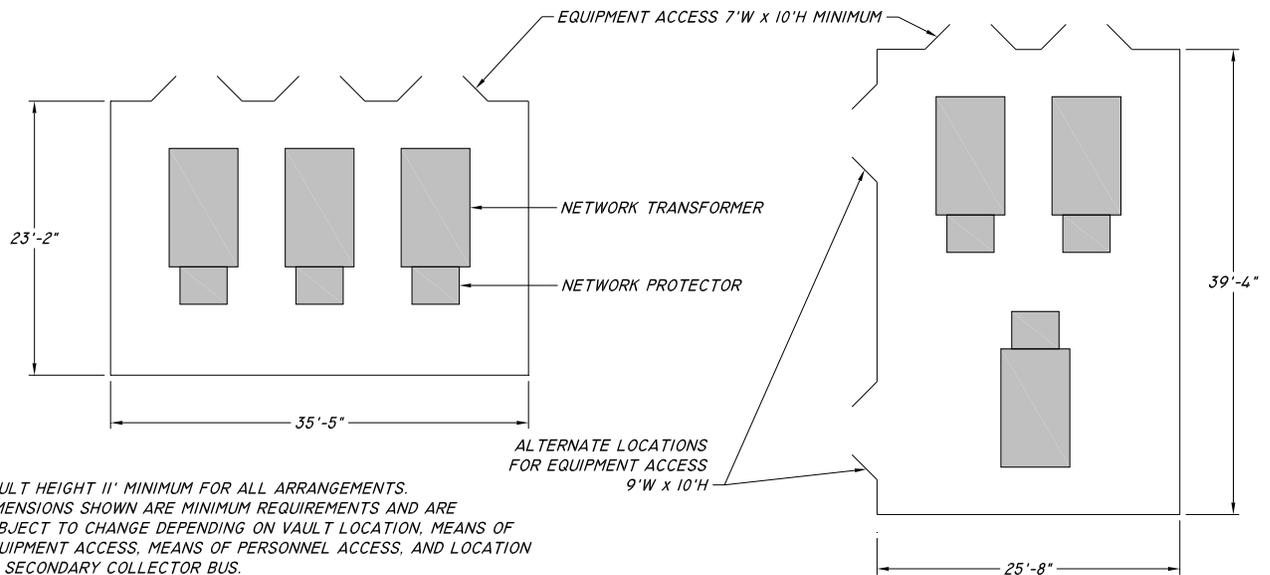
**Figure 27 – Building & Free-Standing Vault Standard Arrangements, 3 – 2500 kVA, 15 kV**
