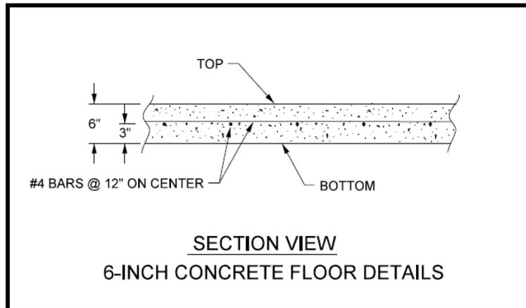
**Figure 55 – Concrete Floor Minimum Standards**
