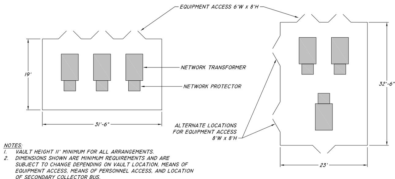
**Figure 18 – Building & Free-Standing Vault Standard Arrangements, 3 – 1000 kVA, 15 kV**
