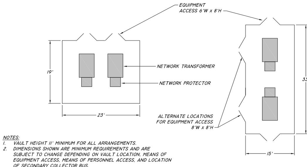
**Figure 17 – Building & Free-Standing Vault Standard Arrangements, 2 – 1000 kVA, 15 kV**
