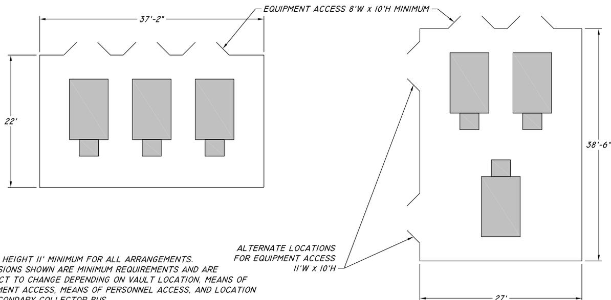
**Figure 45 – Building & Free-Standing Vault Standard Arrangements, 3 – 2000 kVA, 34.5 kV**
