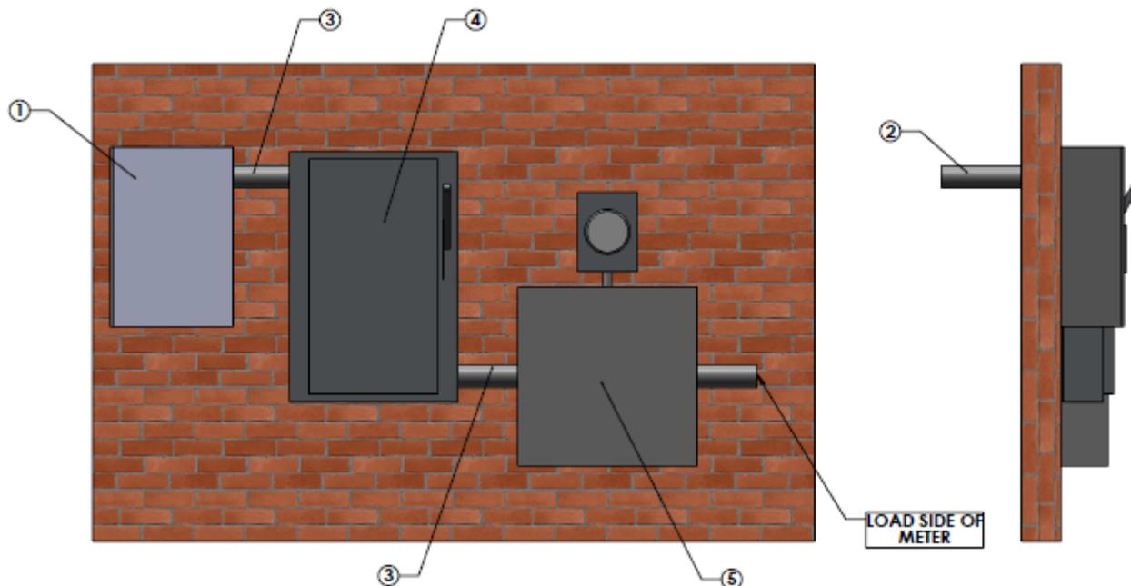
**Figure 7 – 400 amperes Three Phase Equipment Example Layout**
