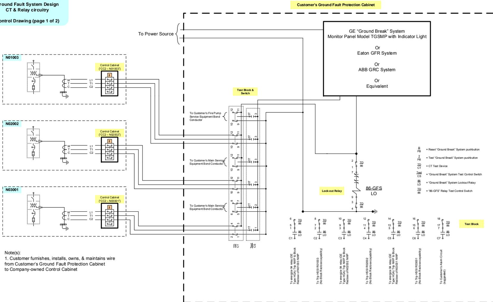
Figure 58 – Ground Fault Protection Control System Example Sheet 1
