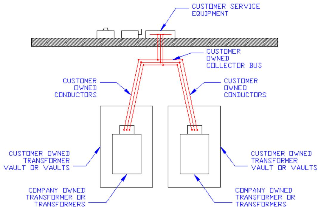
**Figure 16 – Spot Network Customer-Owned Transformer Vaults**
