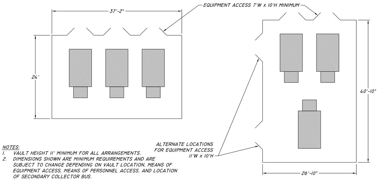
**Figure 39 – Building & Free-Standing Vault Standard Arrangements, 3 – 2500 kVA, 23 kV**
