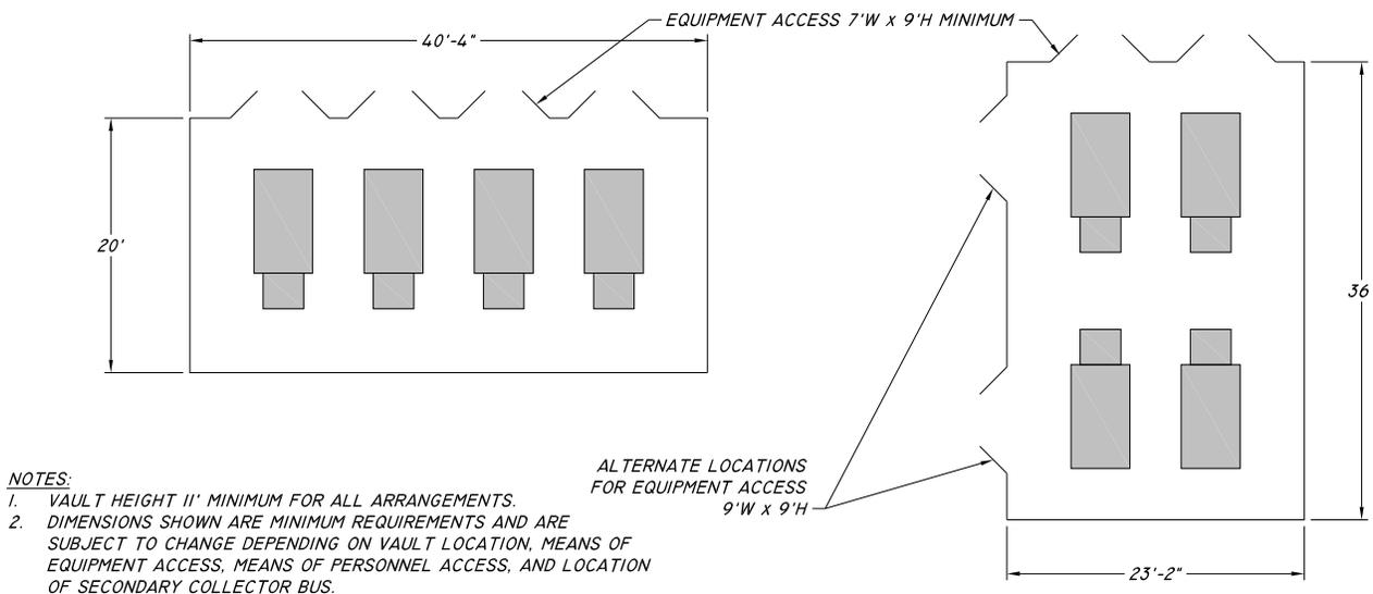
**Figure 31 – Building & Free-Standing Vault Standard Arrangements, 4 – 1000 kVA, 23 kV**
