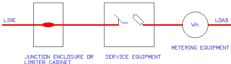
**Figure 1 – Cold Sequence Metering**
