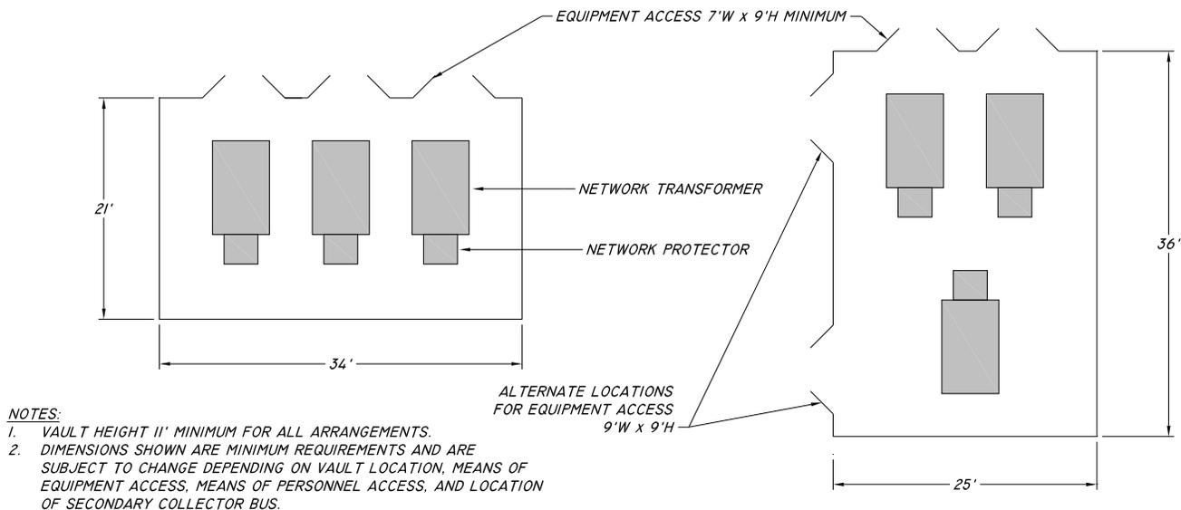
**Figure 24 – Building & Free-Standing Vault Standard Arrangements, 3 – 2000 kVA, 15 kV**
