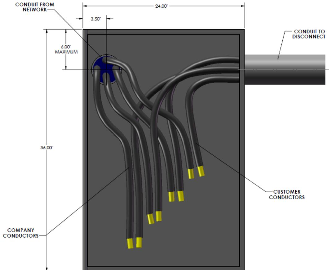
**Figure 8 – 400 ampere Three Phase Junction Enclosure Example Layout with conductors**
