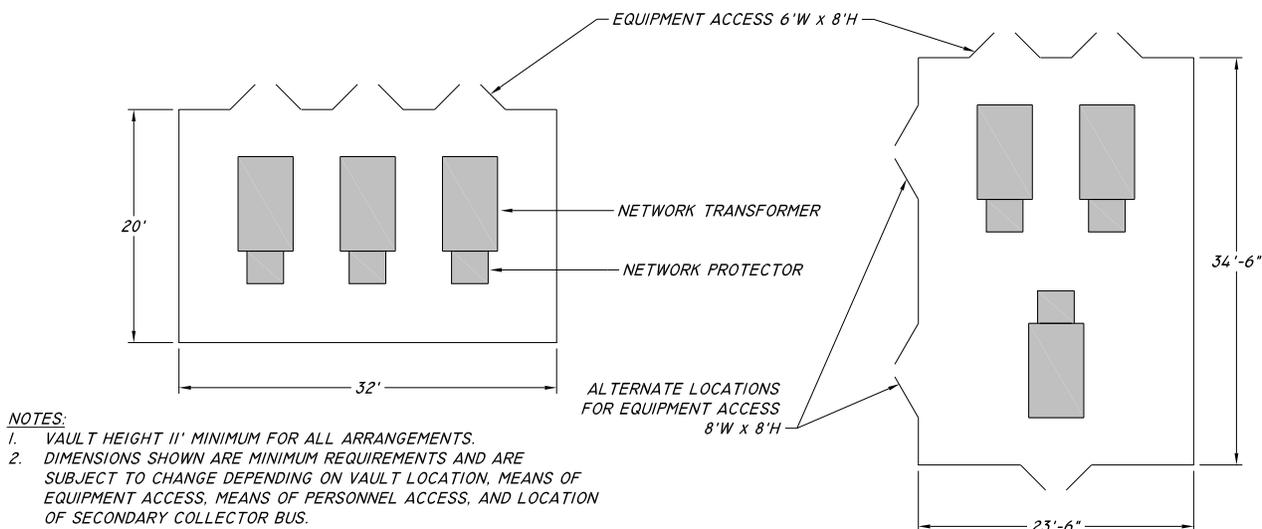
**Figure 21 – Building & Free-Standing Vault Standard Arrangements, 3 – 1500 kVA, 15 kV**
