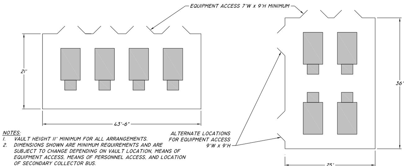
**Figure 25 – Building & Free-Standing Vault Standard Arrangements, 4 – 2000 kVA, 15 kV**
