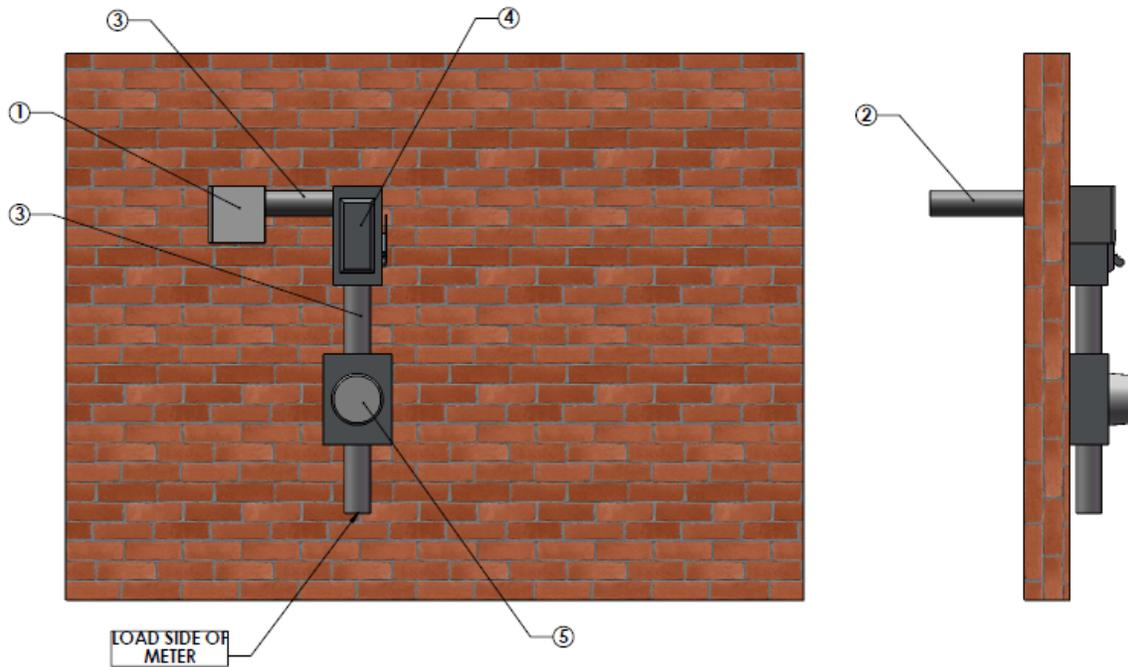
**Figure 3 – 100 to 200 amperes Single Phase Equipment Example Layout**
