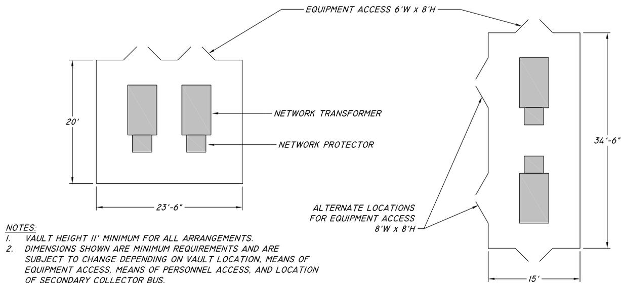
**Figure 20 – Building & Free-Standing Vault Standard Arrangements, 2 – 1500 kVA, 15 kV**
