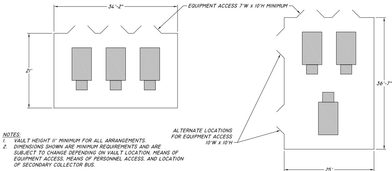
**Figure 42 – Building & Free-Standing Vault Standard Arrangements, 3 – 1500 kVA, 34.5 kV**
