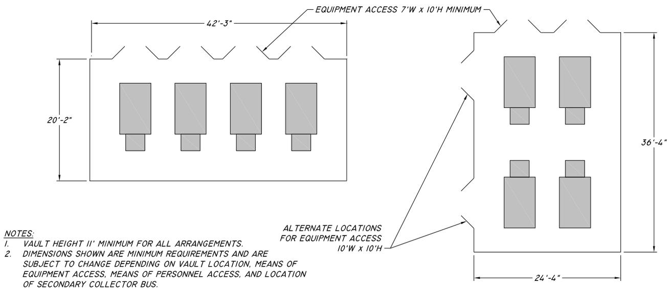
**Figure 34 – Building & Free-Standing Vault Standard Arrangements, 4 – 1500 kVA, 23 kV**
