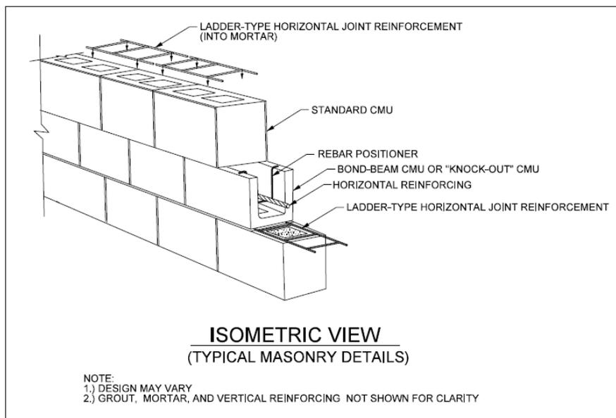
Figure 54 – CMU Wall Minimum Standards Isometric View
