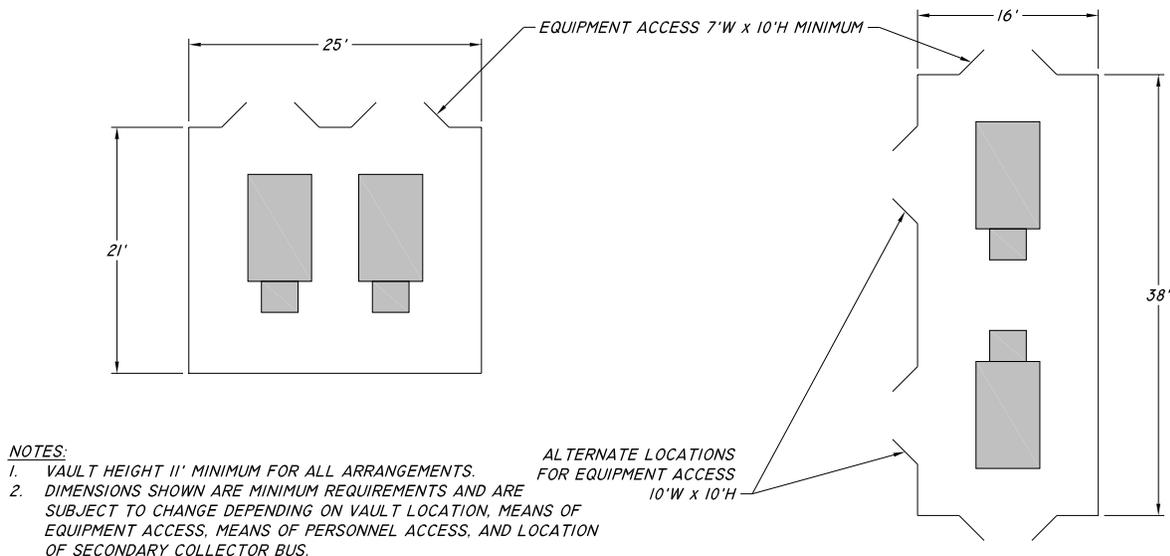
**Figure 41 – Building & Free-Standing Vault Standard Arrangements, 2 – 1500 kVA, 34.5 kV**
