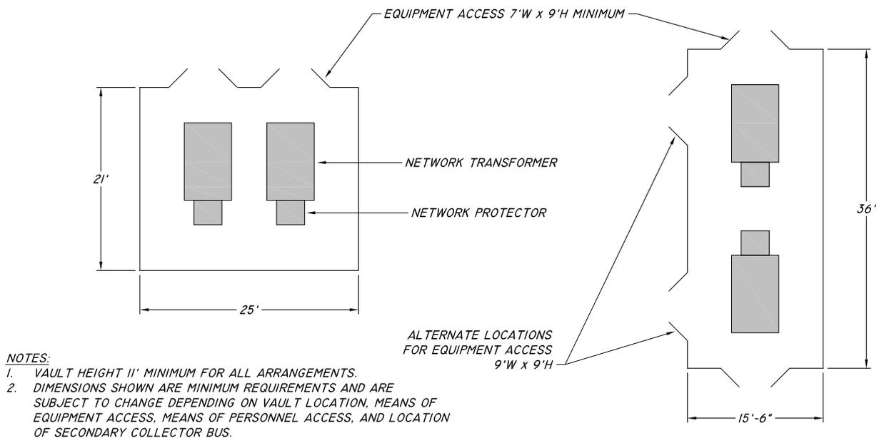
**Figure 23 – Building & Free-Standing Vault Standard Arrangements, 2 – 2000 kVA, 15 kV**
