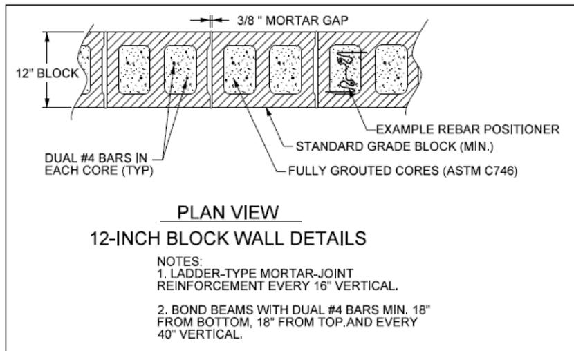
Figure 53 – CMU Wall Minimum Standards Plan View
