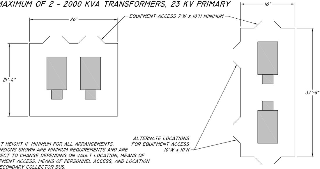
**Figure 35 – Building & Free-Standing Vault Standard Arrangements, 2 – 2000 kVA, 23 kV**
