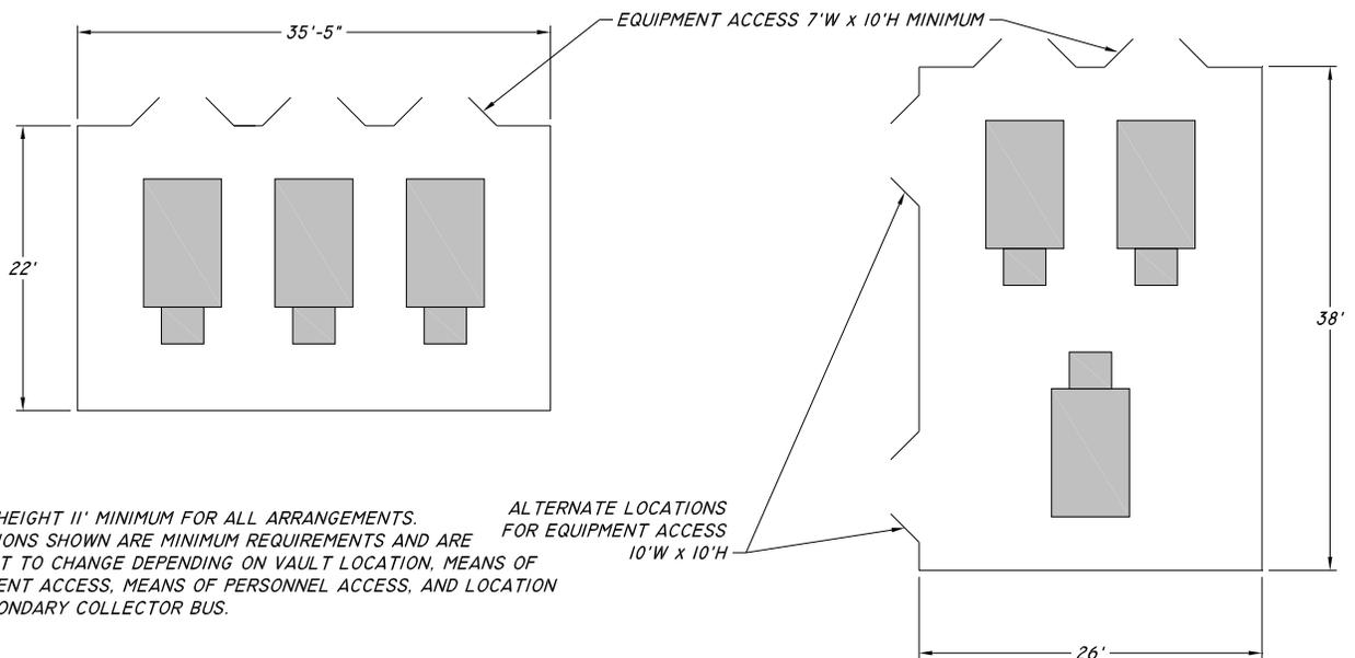
**Figure 36 – Building & Free-Standing Vault Standard Arrangements, 3 – 2000 kVA, 23 kV**
